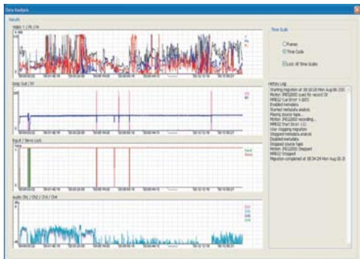
*SAMMA Eye™ generates post-migration color-coded data analysis graphs for video parameters Y/Pb/Pr, as well as for drop-outs, RF, servo-lock and audio.*
